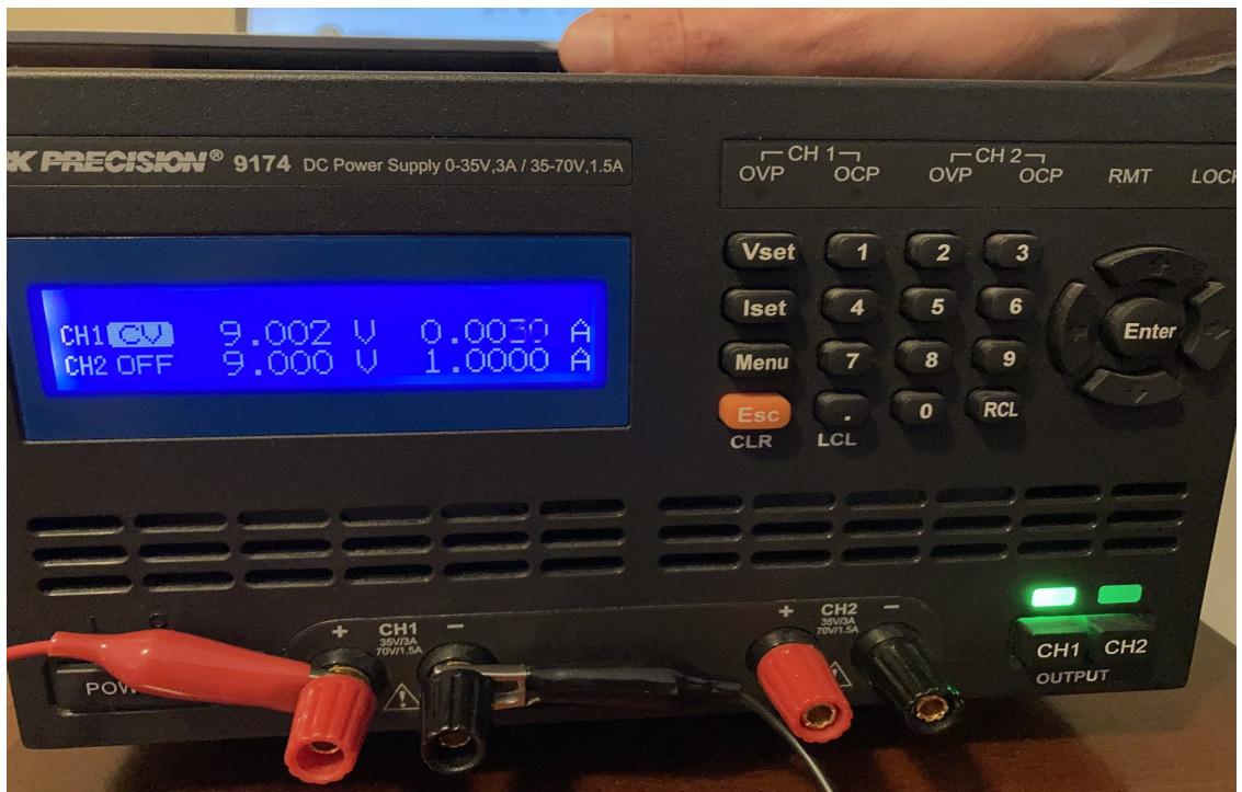
Figure 59: DC Power Supply for Testing (9V, 500mA)
