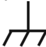
Figure 30: Chassis Ground Symbol
