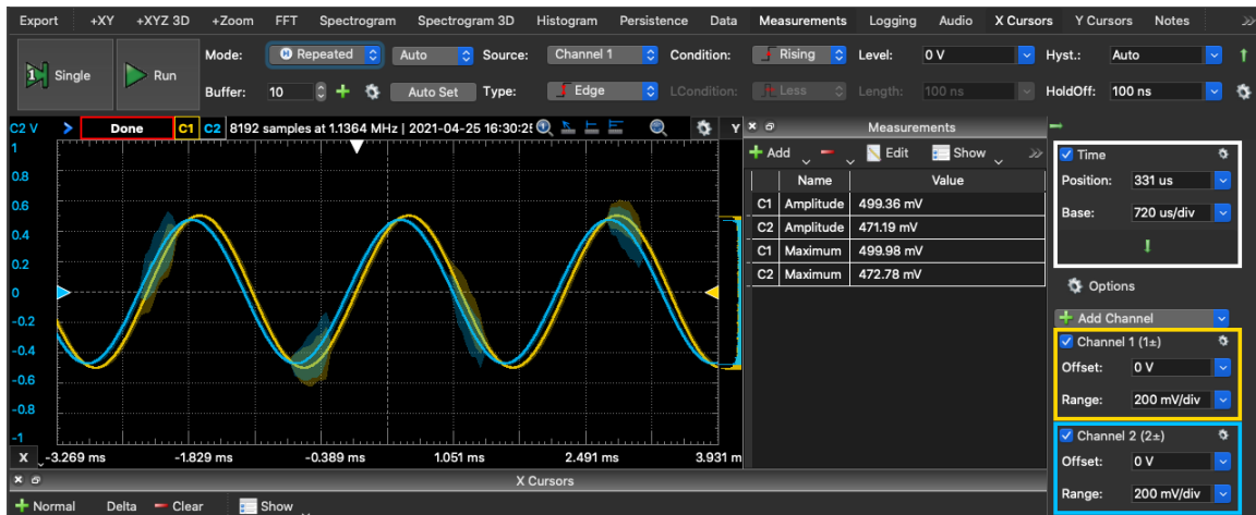
Figure 61: Input Buffer Transient Response ( V_{in} = 500\text{mV} , 440Hz)
